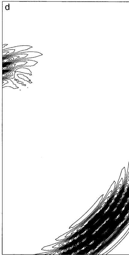
FIG. 8. Test 2, isocurves of the numerical solution at time t = 1.6 ( u_{\min} = -0.235 u_{\max} = 0.215 , \Delta = 0.01 ): (a) first-order Engquist and Majda NRBC; (b) present first-order nonlinear adaptive NRBC; (c) second-order Engquist and Majda NRBC; (d) present second-order nonlinear adaptive NRBC.
